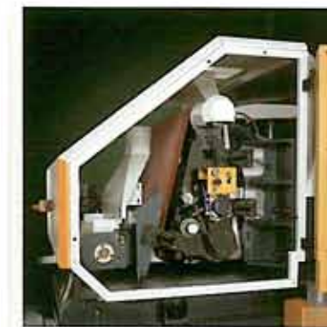
When finish sanding is required, an optional sanding module is installed behind the planing head to get the job done in a single pass. Models are also available to process both bottom and top surfaces of a board or panel in one pass.
